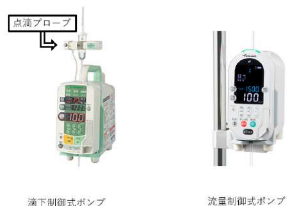
Fig. 3. Example of drop control type infusion pump and peristaltic finger infusion pump
